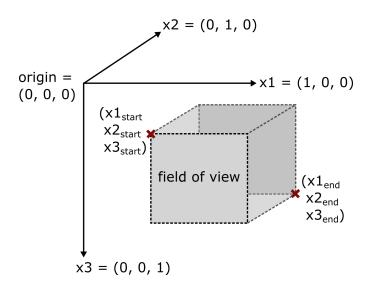
In summary, all coordinate positions of individual elements will be given in cartesian coordinates consistent with the field of view definition of the device. Since the field of view and element positions of the imaging device reside in this same coordinate system, the origin of
