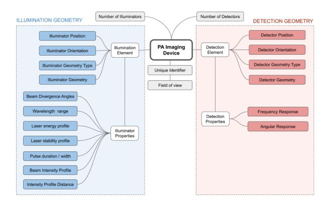
**Figure 2:** Graphical overview of the proposed *Imaging Device Metadata* divided into (1) the illumination geometry and (2) the detection geometry.
